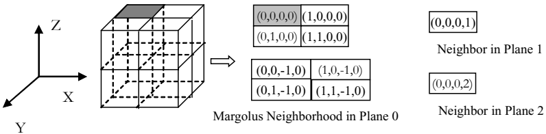
Fig. 6. A cell and its neighborhood definition at the deformation stage
